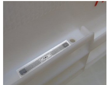
The picture shows the label to be applied underneath the outer rim, the plastic crate is upside down.
